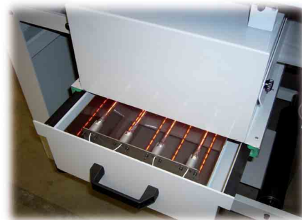
Cassette infra-rouge. Infrared drying unit.
