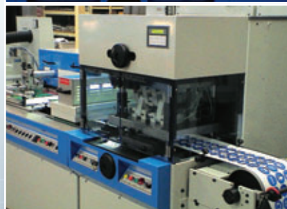
Flat bed die cutting station.
